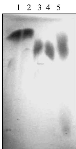
Fig. 3. Thin layer chromatographic profiles of NADH (lane 1); NADPH (lane 2); NADH (heat treated) (lane 3); NADPH (heat treated) (lane 4) and placental extract (lane 5). Solvent was ethanol:water = 90:10.
